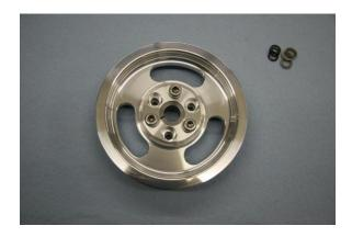
Photo #3 (Location of screws for hub/pulley separation)
