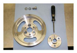
Photo #4 (Using small screwdriver to spread hub slot)
