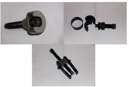
Photo #2 (Sample Pulley Pullers)
